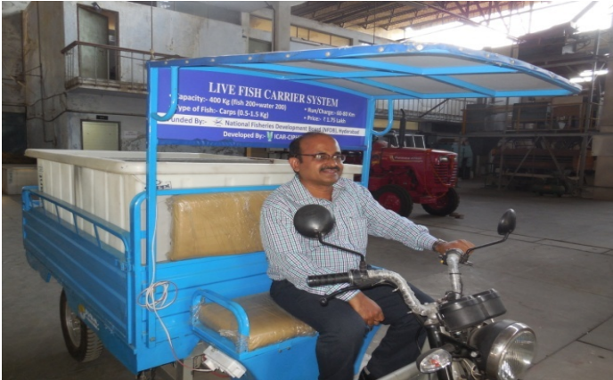
Live-fish carrier system developed by CIPHET, Lucknow with NFDB assistance
